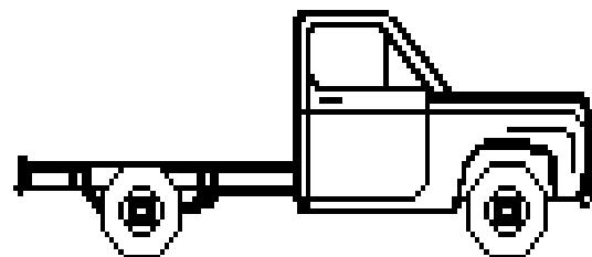
3. **“Chassis Cowl” Cab and Chassis** - Consists of a chassis, engine, front sheet, and fenders, with no cab. This allows for a secondary body, which includes a driver and passenger compartment to be added.
